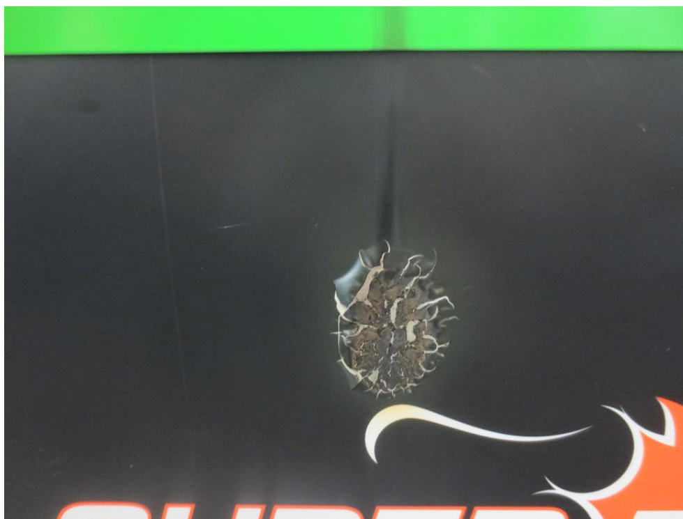
Picture 15 After the flame-retardant test
