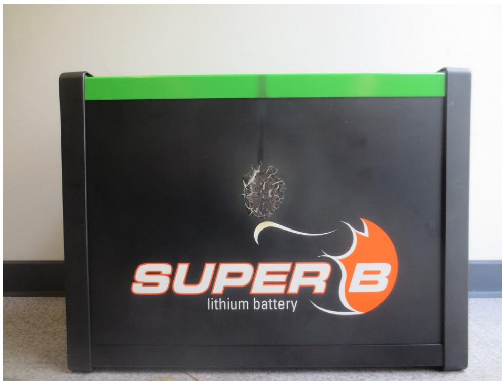
Picture 14 After the flame-retardant test
