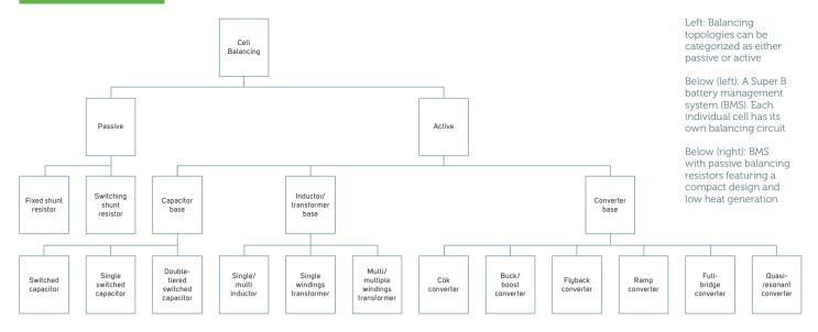
Passive balancing methods remove the excess charge from the more fully charged cell(s) through passive resistors until the charge matches that of the lower cells in the pack or a charge reference. The resistor will be in either fixed mode or switched.
